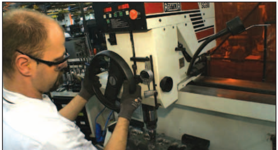
The Rottler SG9M seat and guide machine uses a dead pilot design that stays stationary in the guide as the cutting head rotates around it.
