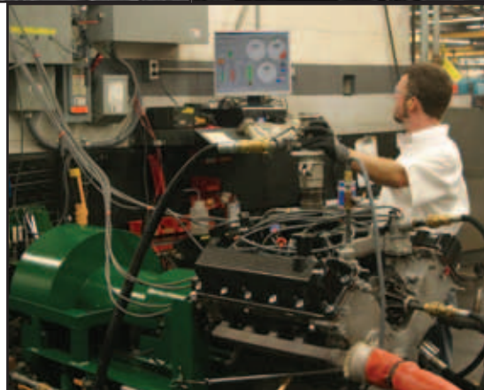
Clockwise from above: Engine remanufacturing at JASPER during the 1950's. We've come a long way since then. Businessman Alvin C. Ruxer started JASPER in 1942 out of necessity during World War II. Using computerized data acquisition to live run test gas engines, JASPER is a recognized leader in remanufactured products.
