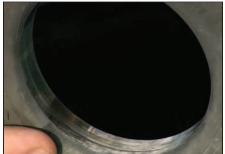
Figure 1 - The lock-up piston of the 47RE/48RE will wear on one side of the inner seal but not on the other. JASPER eliminates the wear issue by centering a sleeve kit to the damper assembly.
