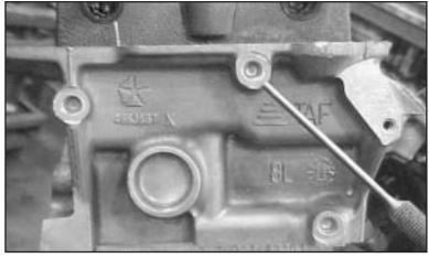
JASPER's New Product Group noticed oil leaking from the plugs in the cylinder heads of the Chrysler 2.7 liter V6.
