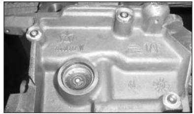
JASPER drills, taps and plugs the Chrysler 2.7 liter heads to eliminate the chance of oil leaks.
