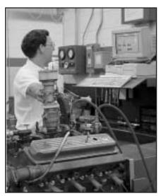
Final preparations are made to the engine before the computer test begins.
