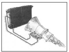
This is the setup for a typical oil-towater transmission cooler
