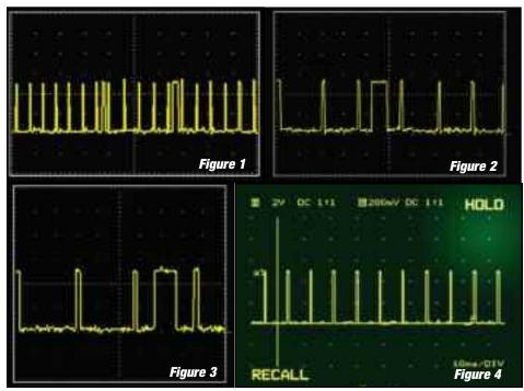
The rough-running Jeep Cherokee showed this type of wave pattern when hooked up to the scope (figures 1, 2 & 3). These images were compared to a known good pattern (figure 4).
