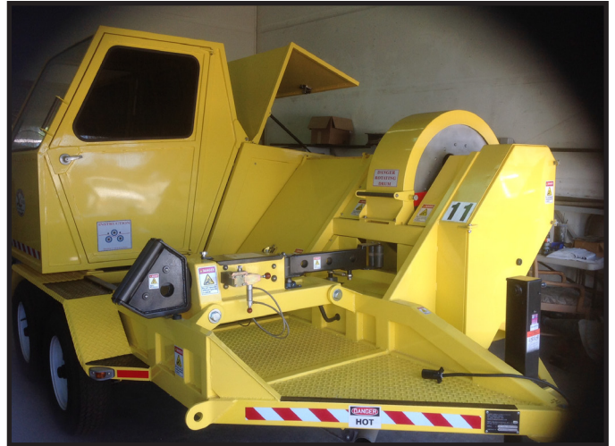
This 6,700 pound glider launching winch from Roman's Design can propel a glider into the sky at speeds over 80 mph.
