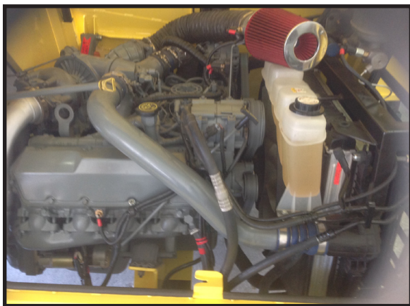
A 325 horsepower JASPER 7.3L International diesel engine turns the winch that helps the glider take flight.
