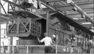
Process times for JASPER's Kolene salt bath have been adjusted for the most efficient cleaning and thorough removal of contaminants.
