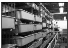
A 58' long computerized carousel holds up to 88 transmissions ready for final assembly.
