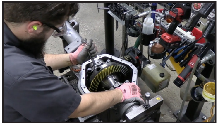
Tooth contact pattern is checked as the ring and pinion gears are worked back and forth against a yellow marking compound.
